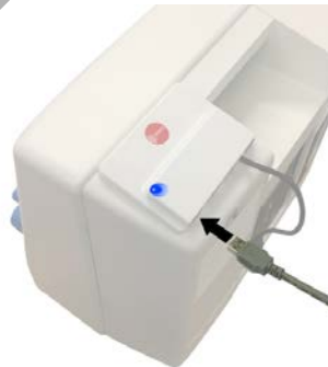
Figure 10.1.6. connecting the PhysioFlow Q-Link.
