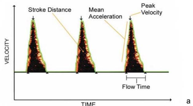
**Figure 8.** Waveform displaying Stroke Distance, Peak Velocity, Mean Acceleration and Flow Time measurements
