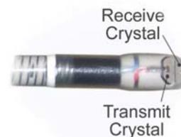
**Figure 5.** Receive and transmit ultrasound piezo-electric crystals
